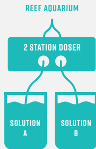
Two station dosing setup example.
